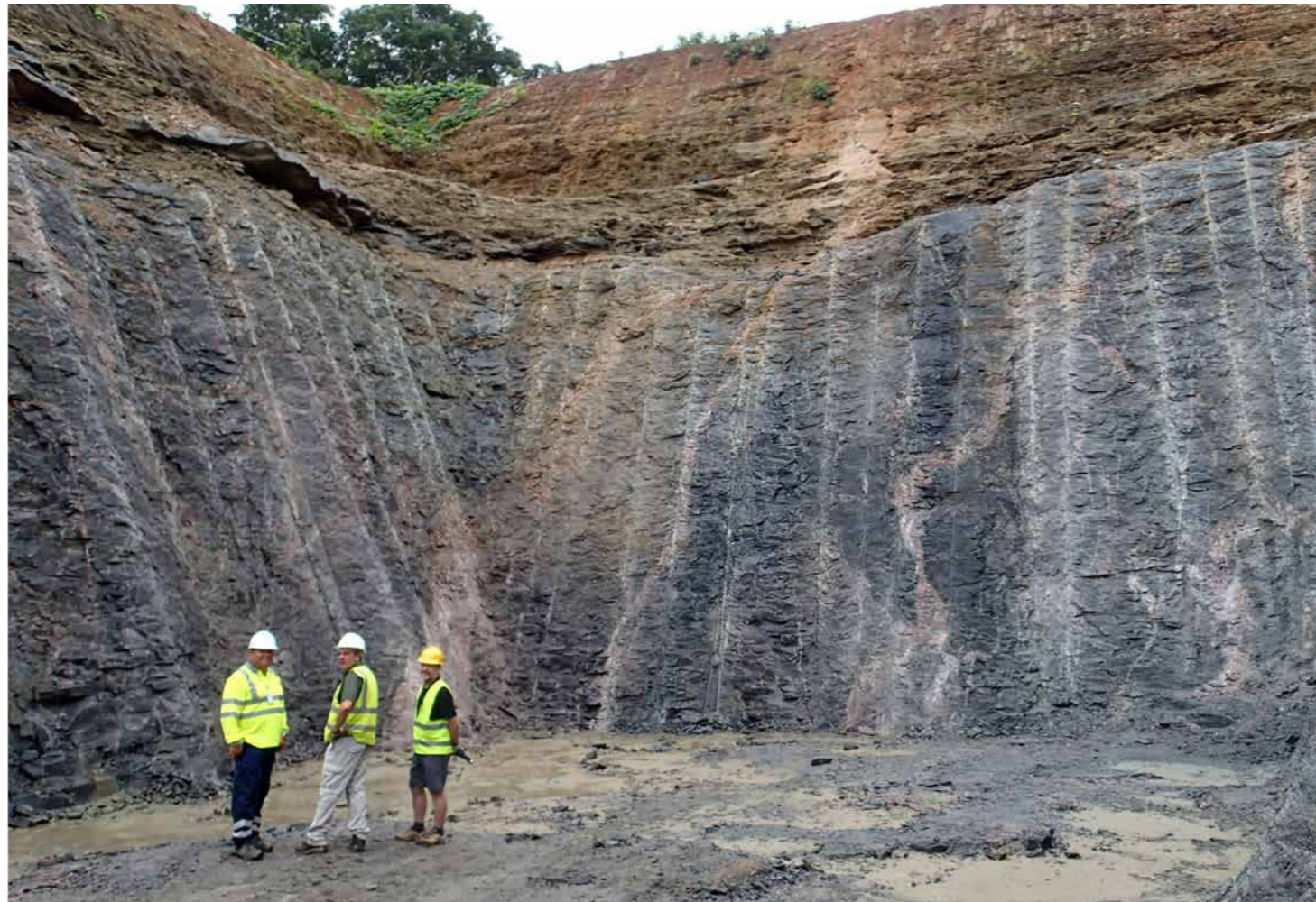
^ L-R. Tongo Management Team, Pre Split and Bench 1 drill pattern and Boxcut brow with Max Wessie
